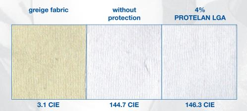
Phenolic yellowing test M&S C20B
